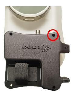
Use the 2 M3x15 CHC screws supplied to mount the bracket under the T-Box (under the battery and antenna).
