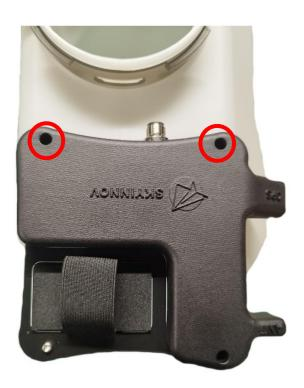
Drill 3.5 mm holes in the tank in the positions marked out above.
