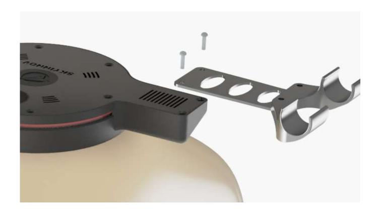
Remove the two M3x6 FHC screws under the screen and replace them with the two M3x10 BHC screws provided to secure the carbon plate of the bottom bracket.
