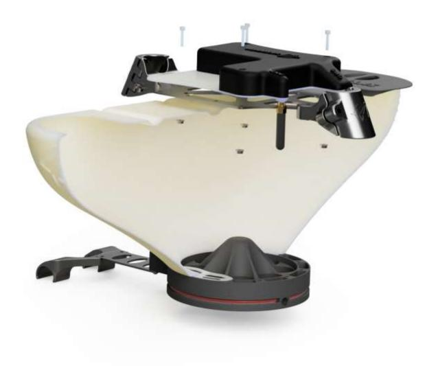
Use the 4 supplied M3x15 CHC screws to mount the T-Box to the spreader tray by sandwiching the carbon plate of the bracket.
