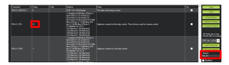
RELAY\_PIN is set to "51" since the DROP cable is connected to aux2 / pin51.
