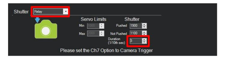
The trigger type is set to "Relay" to have a control pulse (I/O mode) and a pulse duration of 3/10 of a second.
